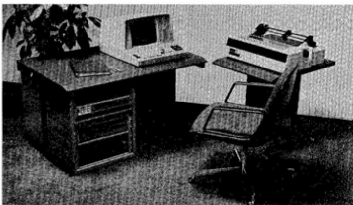
PERTEC COMPUTER CORPORATION's new MITS 300 Business System is comprised of a mainframe, a CRT terminal on a desk, and a line printer on a pedestal. Pictured here is the MITS 300/55, which is the hard disk, rather than the floppy disk, system.
